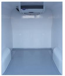
High thermal efficiency 'one piece moulded panels' for roof, side's bulkhead and floor
